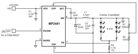
Figure 4—Step-up/down White LED Driver Application
