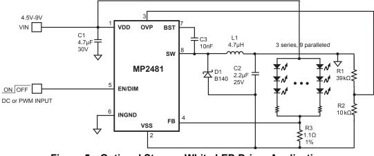
Figure 5—Optional Step-up White LED Driver Application
